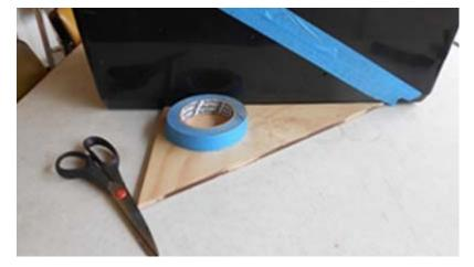
2a Use a 30 degree angle template to mark the position.
