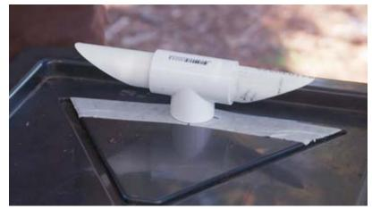
**1d** Cut coupling in half. Cut another short piece of pipe at 45mm pipe and attach to the bottom of the tee. Use coupling to attach to the lid. One piece of coupling is flush to the underside of the lid.
