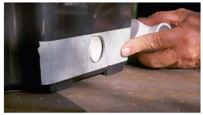
**3b** Install a pipe at the bottom of the storage box to provide a means for the juice to exit.
