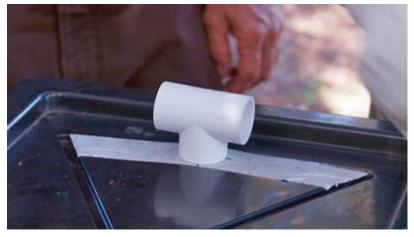
**1c** Cut two sections of 100mm pipe, then cut one end at angle (30 degrees) as this will encourage fly to enter. Attach pipe segments to each end of the PVC tee with a screw.
