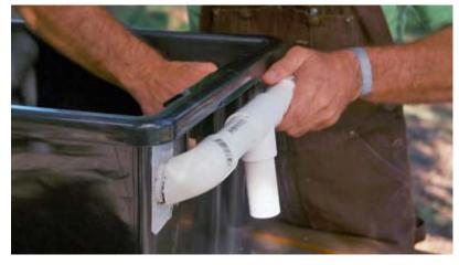
**2f** Attach to central PVC Tee which allows the larvae to emerge to fall into a strategically placed container.
